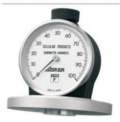
The ASKER Durometer Type F for much softer specimens (low hardness) gives accurate readings as it features a larger indentor and pressure foot.
