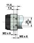
Mounting: rope outlet sideways bottom (S2), rope outlet bottom (S3) Sensors with option rope outlet S2 and S3 have a modified base plate:
