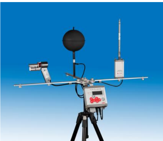
M-Log (ELO009) tripod mounting using a stand.
